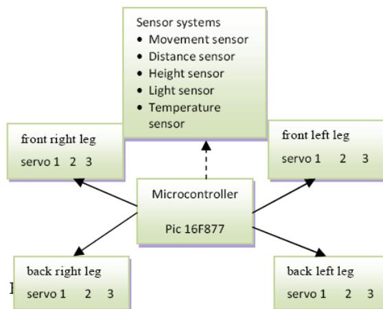
**Figure 5:** electronic design block diagram of the spiderbot.
