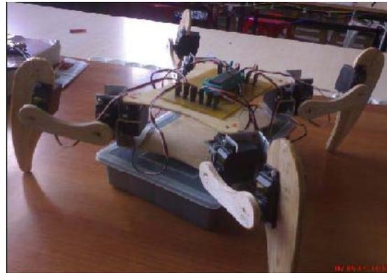
**Figure 3:** The appearance of all the mechanical structure of spiderbot.
