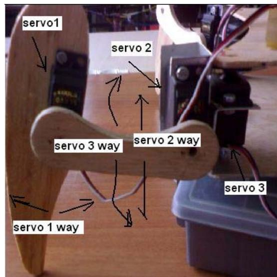
**Figure 4:** The movement direction of the servo motors
