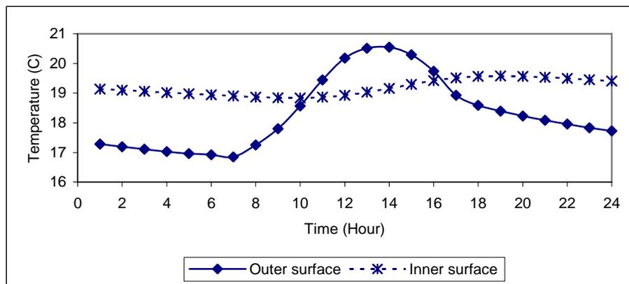
Figure 2. Hourly variation of thermal behaviour of transparently insulated wall
